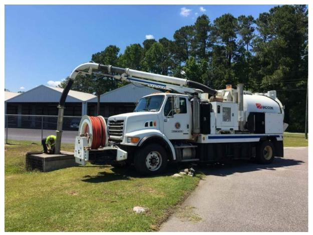
Figure 3-7: Catch Basin Maintenance Operation
